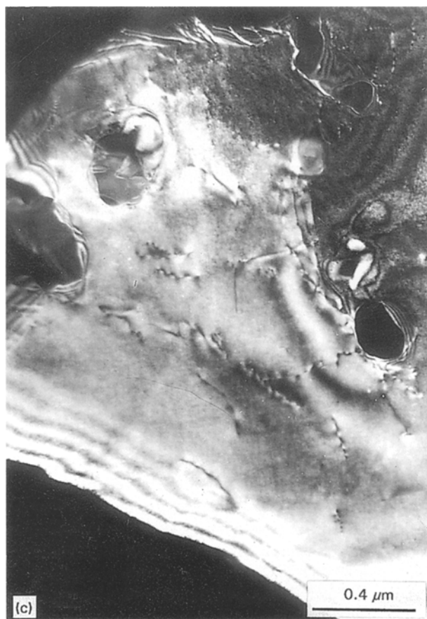
Figure 2 TEM micrographs of HPRS NiAl (a) bright field, (b) selected area electron diffraction (SAED) pattern of the matrix, \beta -NiAl [01 3] zone and (c) dark field of \beta -NiAl corresponding to (a).
