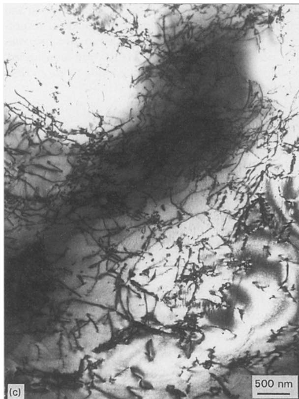
Figure 5 Dislocations in HPRS NiAl (a) dislocation networks among \text{Al}_2\text{O}_3 particles, (b) dislocations bowing out the networks (marked by arrows) and dislocation generation from interfaces between the particle and matrix and (c) dislocations with a high density within the grain.
